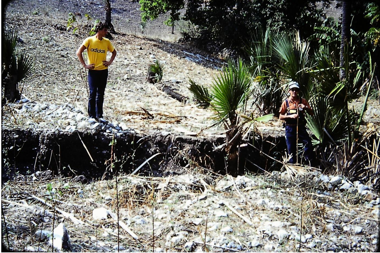
Fig. 58: Field photo from the original 35 mm slide #644 (George Plafker USGS Archive) showing the surface rupture and offset of wall 1 measured on April 20, 1976 as 340 cm of left-lateral strike slip and 83 cm of vertical slip. The view is toward the north.
