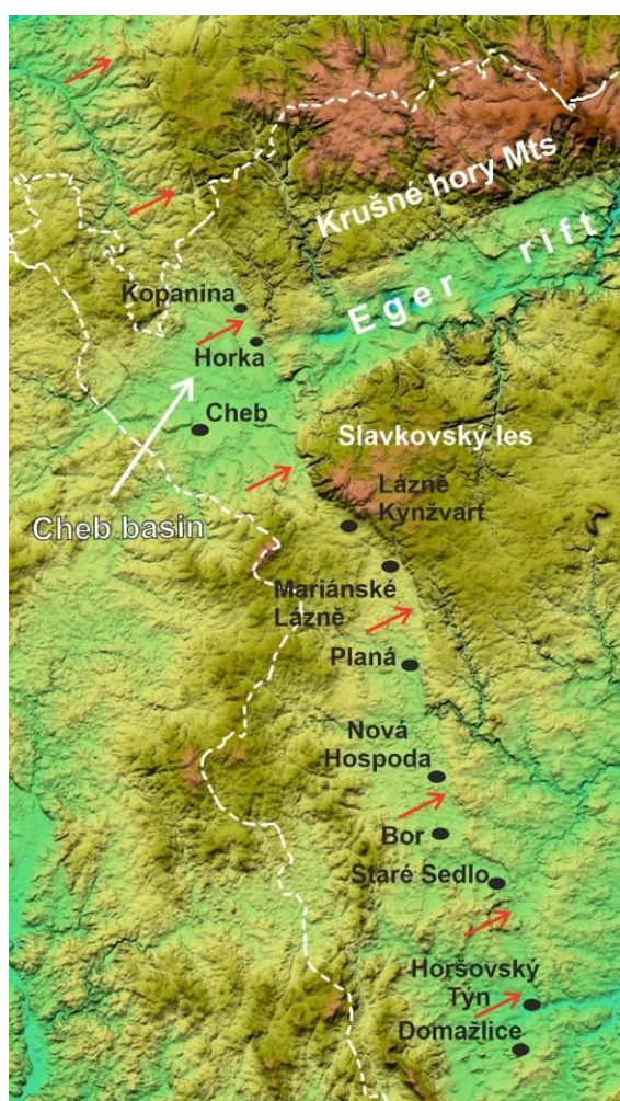
Figure 1: Digital elevation model showing the striking morphology along the Mariánské Lázně fault - pointed by red arrows.
