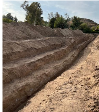
Figure 3: View to the NW of the northern ~130 m (425 ft) of the W wall of the trench showing ~1.5-m-high benches, level line and stations (in feet) on the bottom bench. The dark soil horizon near the level line is the main subject of this paper. The E wall is logged in detail.
