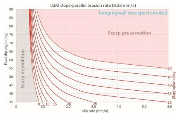
Figure 7: Diagram showing the shift in the scarp preservation-demolition boundary across various fault-slope geometries and slip rate, assuming a constant erosion rate and a transport-limited hanging wall.
