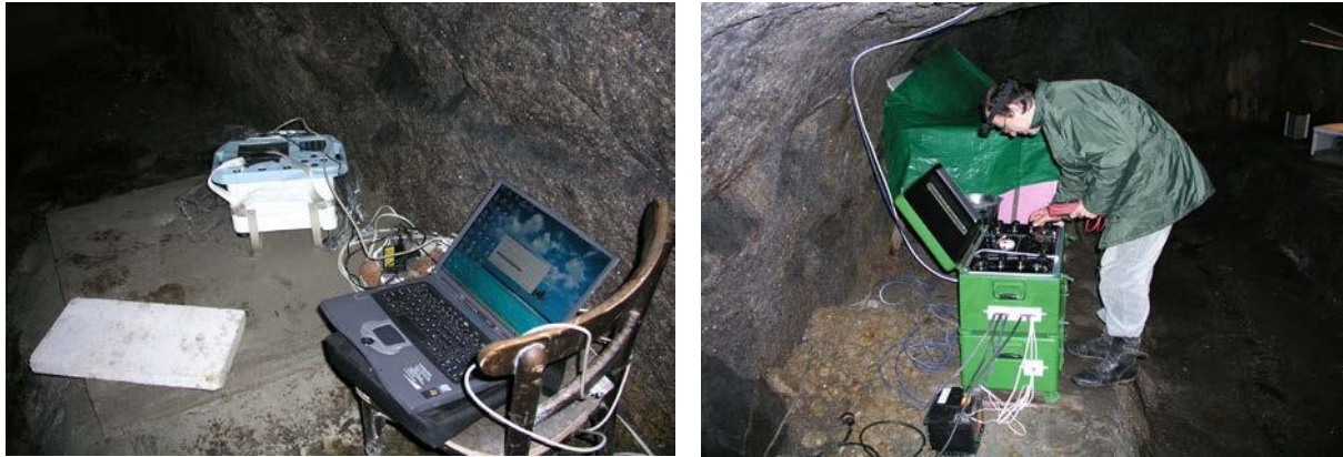
Fig. 31: Gravimeter Graviton EG during data transfer (left), and the recording unit of tiltmeters (right). The tiltmeters are covered by plastic sheets.
