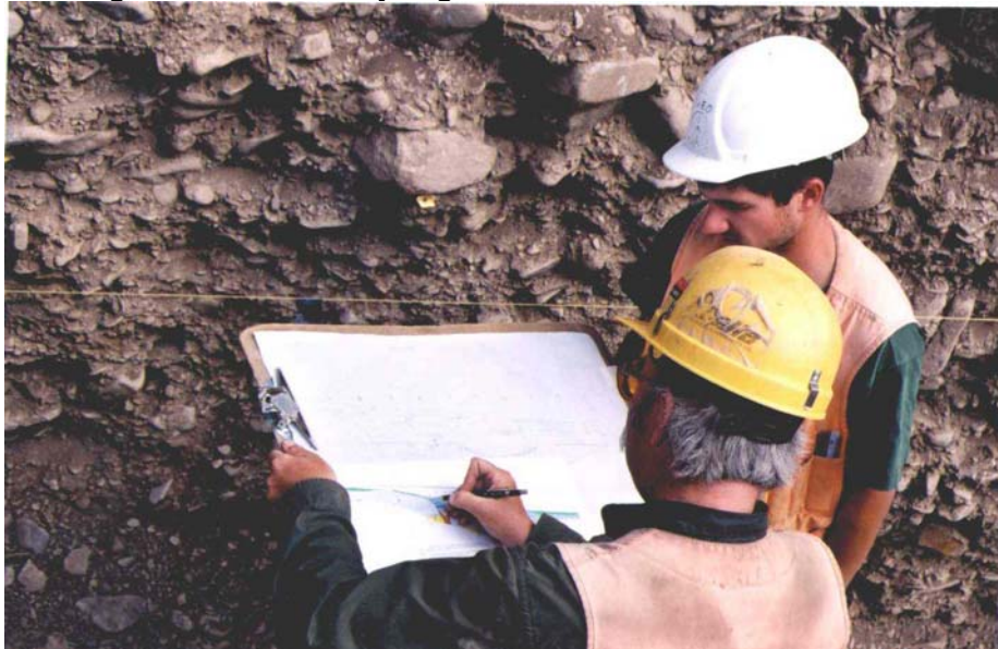
Fig. 3-1. When all else fails, you can make a trench log with manual mapping on graph paper. This 2D technique is the least orthographic and georeferenced of all techniques, but is still the best for showing the critical geologic contacts that define the sequence of events, which is the whole point of trenching. Planimetric precision and accuracy are less important, because if the trench were located several meters in either direction along strike, those values would likely be different. But the number of displacement events and their ages would remain the same, and that is the paleoseismic “story.”
