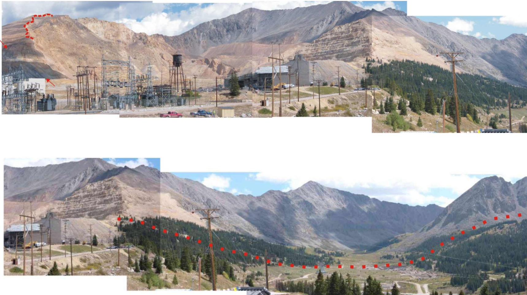
Fig. 9-4. Panoramic photographs of the Climax Mine from Fremont Pass. UPPER PHOTO: the Climax Mine, looking east. The Mosquito fault is exposed between the red arrows at far left. The red dashed line is at the top of the gravitational collapse scarp on Bartlett Mountain. LOWER PHOTO: a continuation of the upper photo, looking to the south. The Mosquito fault (red dotted line) crosses the glaciated valley of the East Fork Arkansas River, and then continues SW at the base of the steep Precambrian range front.
